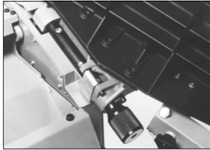
With planing beds in upright position check that safety latches are in position, preventing the inadvertent closing of the tables.
